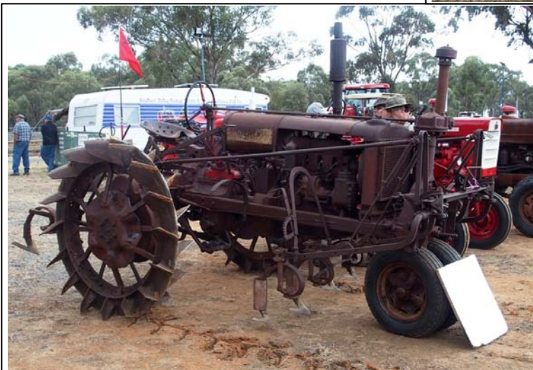
↓ 1938 FARMALL F-20 tractor Fitted with underbelly cultivators with mechanical lift. The original owner, Jake Pederson from Kingaroy, designed and made the rear wheels.
